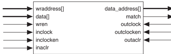
Figure 23. APEX 20KE CAM Block Diagram
